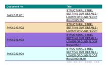
In the above example the architect has used a project number of **1443** followed by **(G10)** to separate out all the *Steel Setting Out* drawings.
